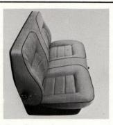
Bench type front seat The Volvo 164 is also available in the form of a version with a bench front seat in combination with steering column gear shift.
